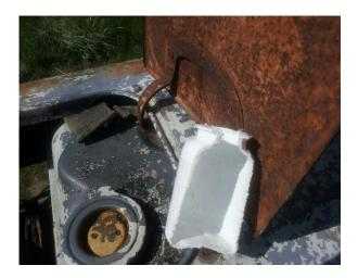
4. You may have to use heat gun (or other heat source) to soften neck of bottle enough to form it into a smaller size, grasping battery cable for secure fitment.
